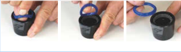
Illustration 246 : Retirer le joint anti-poussière
