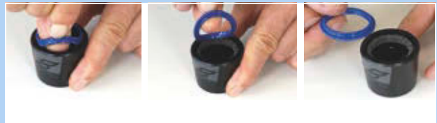
Illustration 211 : Retirer le joint anti-poussière
