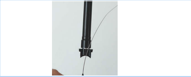
Figure 208: Pulling the end cap out
