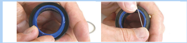
Figure 250: Inserting and fastening the wiper
