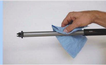
Figure 254: Cleaning the longitudinal groove
