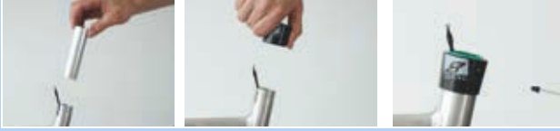
Figure 258: Fitting the slide bushing and outer sleeve
