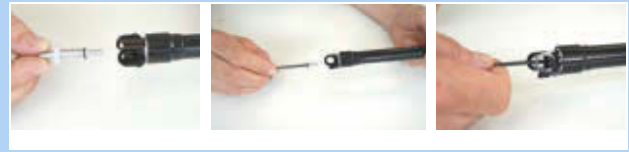
Figure 224: Fastening the cartridge valve cover
